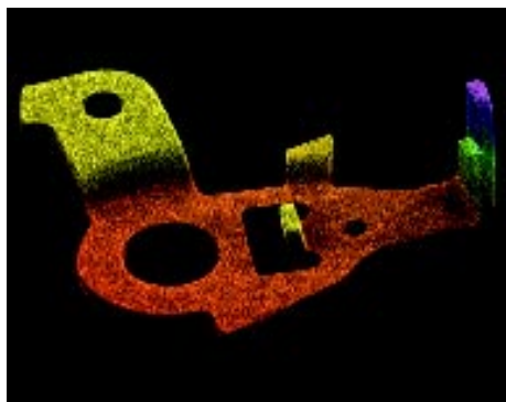
Fig. 3: Point cloud of a metallic probe, colour indicate height.
