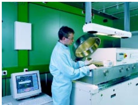
Fig. 1: The magnetron sputtering system Kenotec MRC 903.
